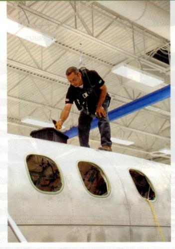
takes components shipped from Brazil, then assembles them using remote-control, laser-guided technology. If working high up, workers are tethered to protect them against falls (left). Mating the wings to the
