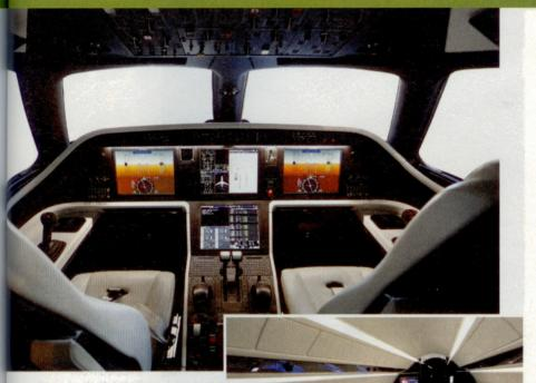
NEXT ON DECK is the Legacy 500, with its fly-by-wire control system, and Rockwell Collins Pro Line Fusion avionics (above). The Legacy 500 cabin (right) promises to redefine the mid-sized category, with its flat floor, six-foot, 10-inch-width, and six-foot-high dimensions. The cabin can be ordered with up to 12 seats. An aft, three-place divan is an option.
